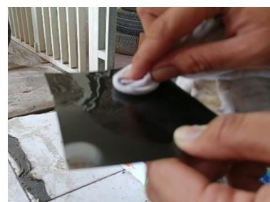
Fig. 2. Gasoline resistance testing
